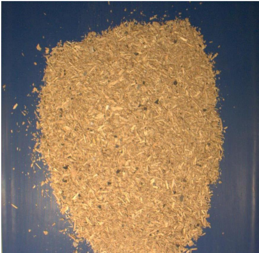
Figure 7: RGB image of a wood chip pile from a shredded painted wood slab. The coated wood chips are distinguished.
