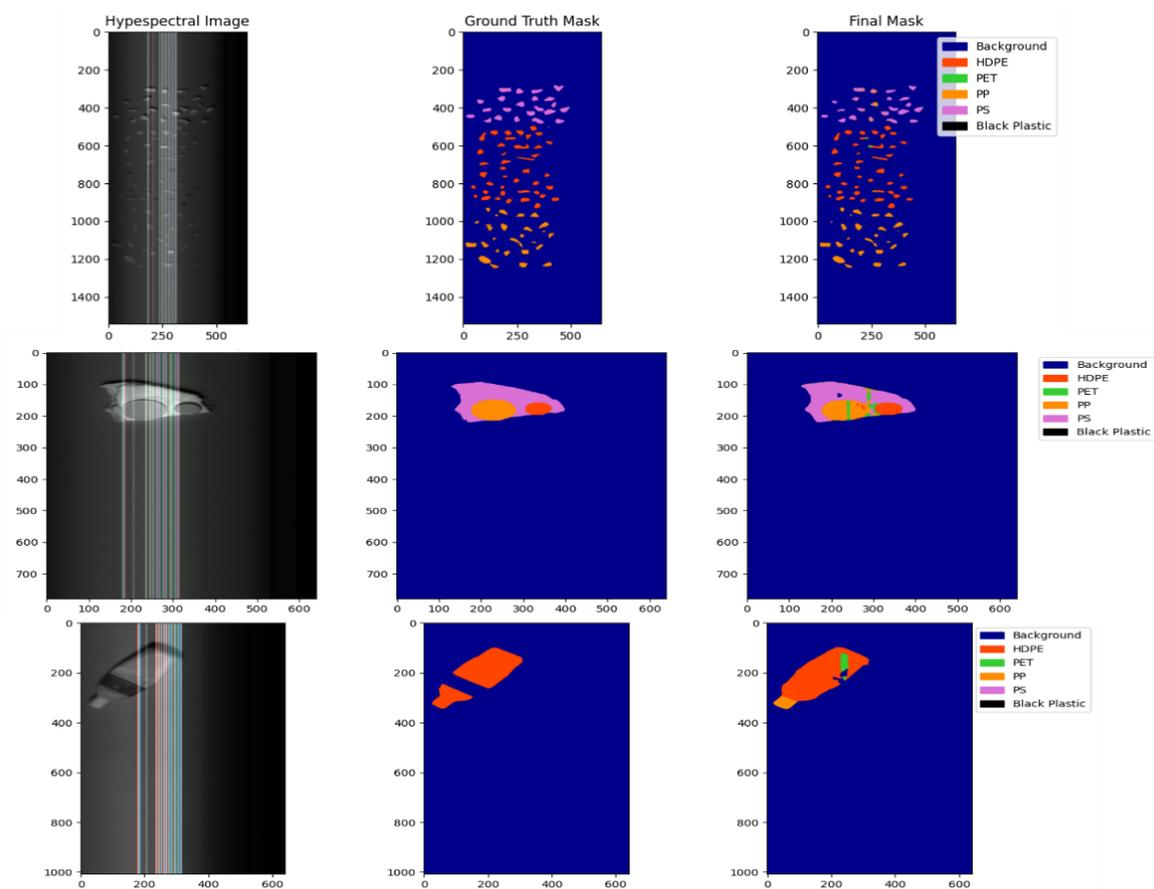
Figure 10: Hyperspectral imaging of plastic samples and visualisation of the CNN-based classifier.
