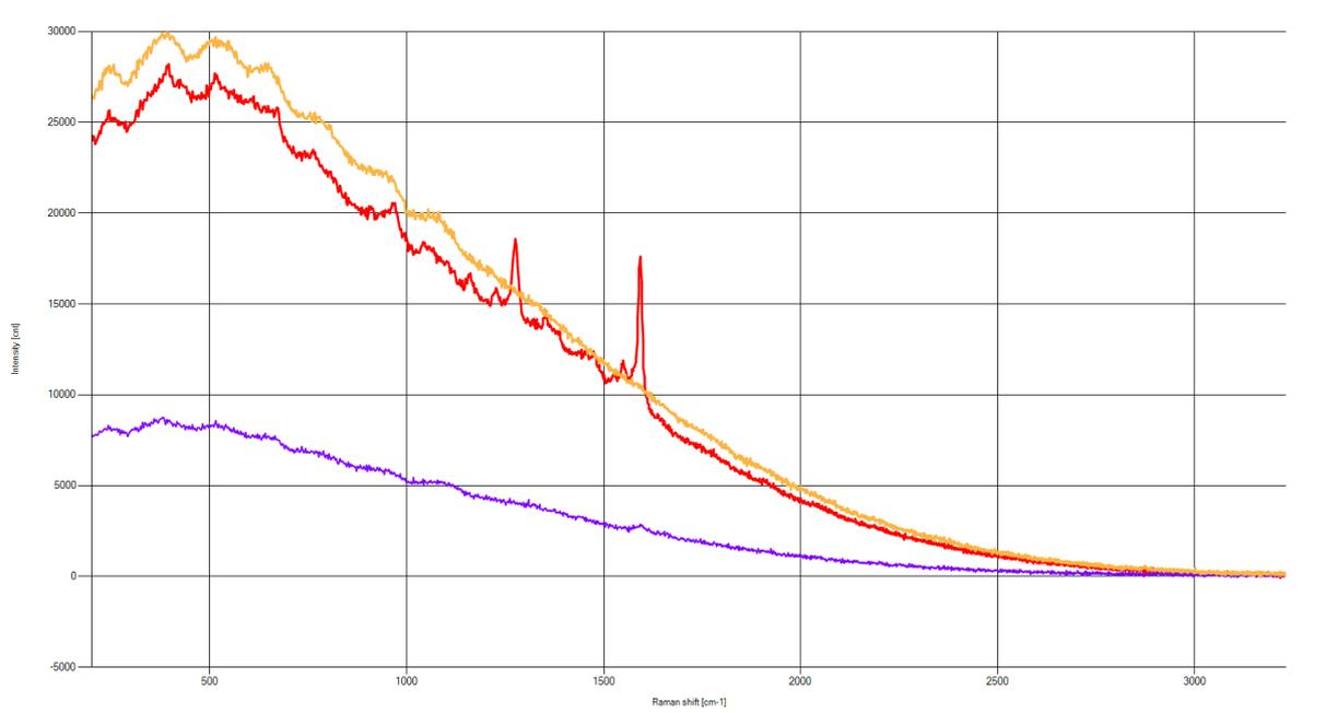
Figure 8: Raman Spectroscopy Intensity for coted wood chip (red), uncoated wood chip from painted wood plank (yellow) and a clean wood chip (blue)
