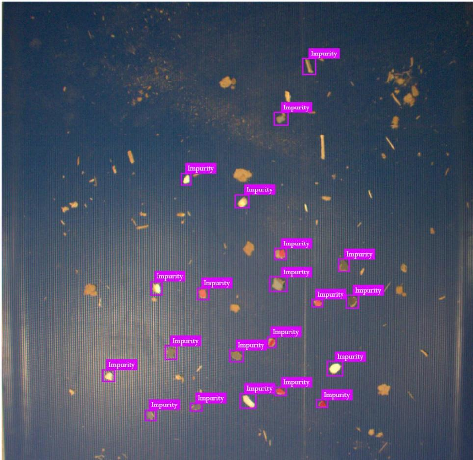
Figure 6: RGB image of a wood chip pile from a shredded painted wood slab classified by fine-tuned YOLO v8 model.
