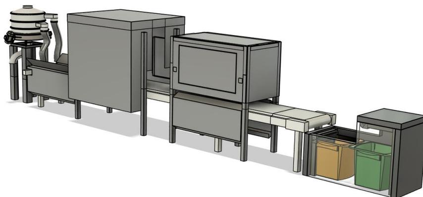
Figure 4: Overall Schematic of the Wood Sorter Design and Workflow
