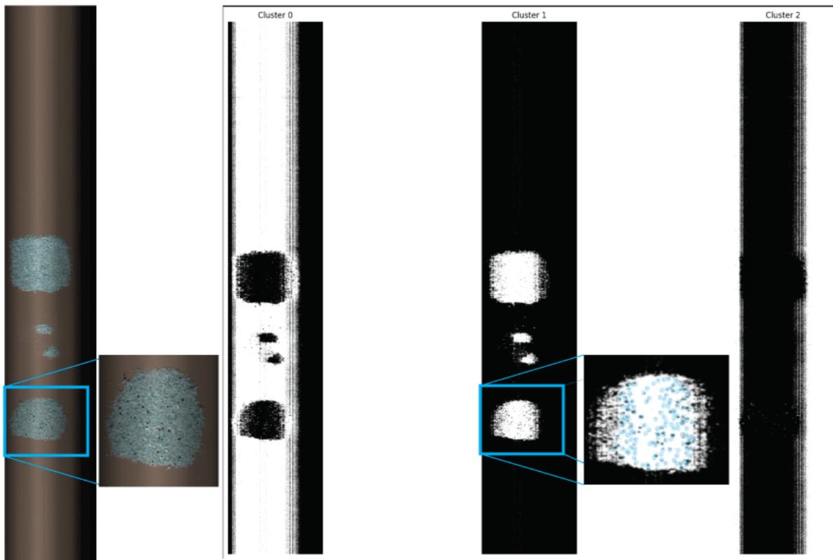
Figure 9: Hyperspectral imaging of impurities and clean wood chips. The identification of impurities is apparent using the kNN clustering algorithm.
