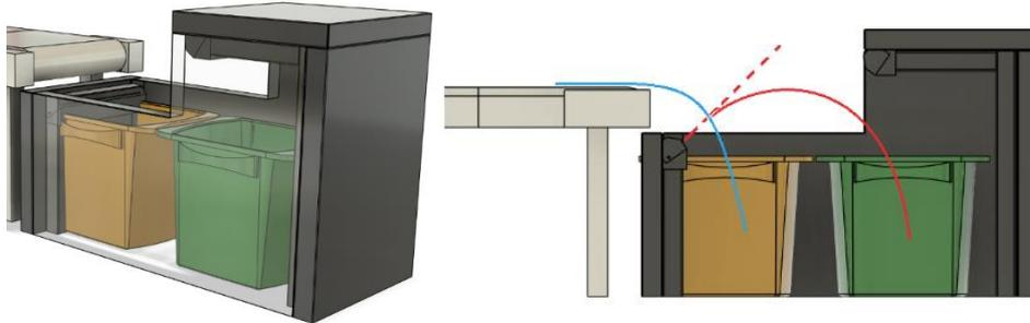
Figure 2: Schematic of Pneumatic Air Nozzles in action
