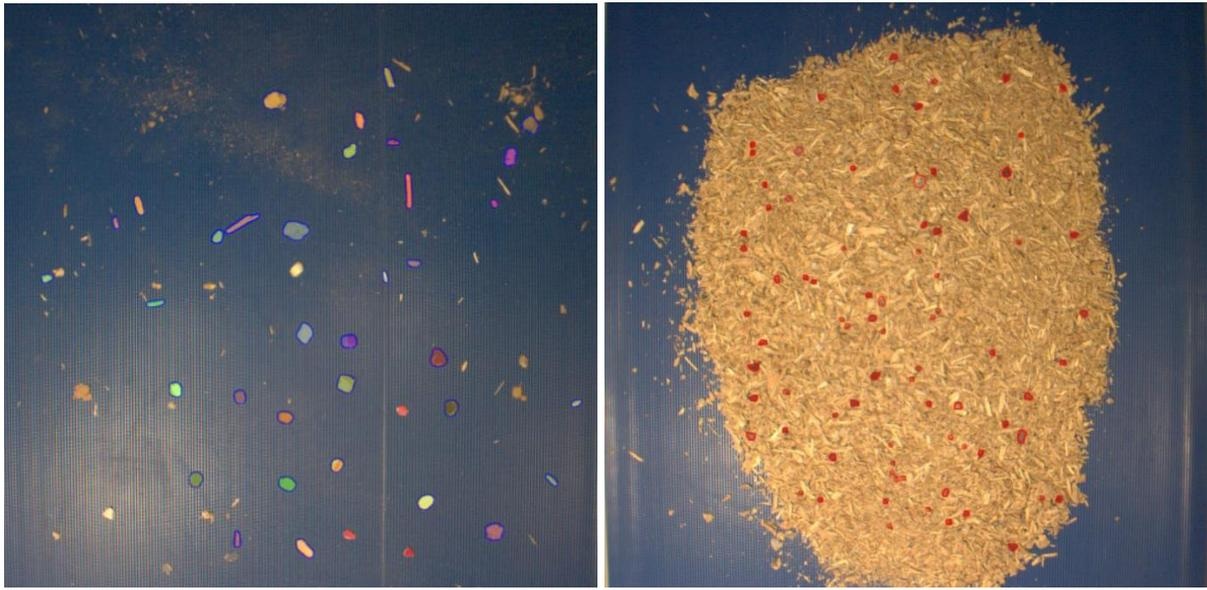
Figure 5: RGB image of a wood chip pile from a shredded painted wood slab segmented by untrained Segment Anything Model.
